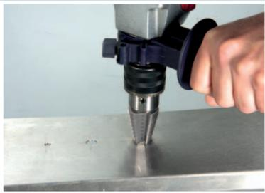
These bits are designed with the capacity to drill multiple hole sizes at once. The bit diameter of these bit types increases from the tip in specific increments following a stair-step profile – like a pyramid, each tier of the bit drills a hole with a different, larger diameter.
